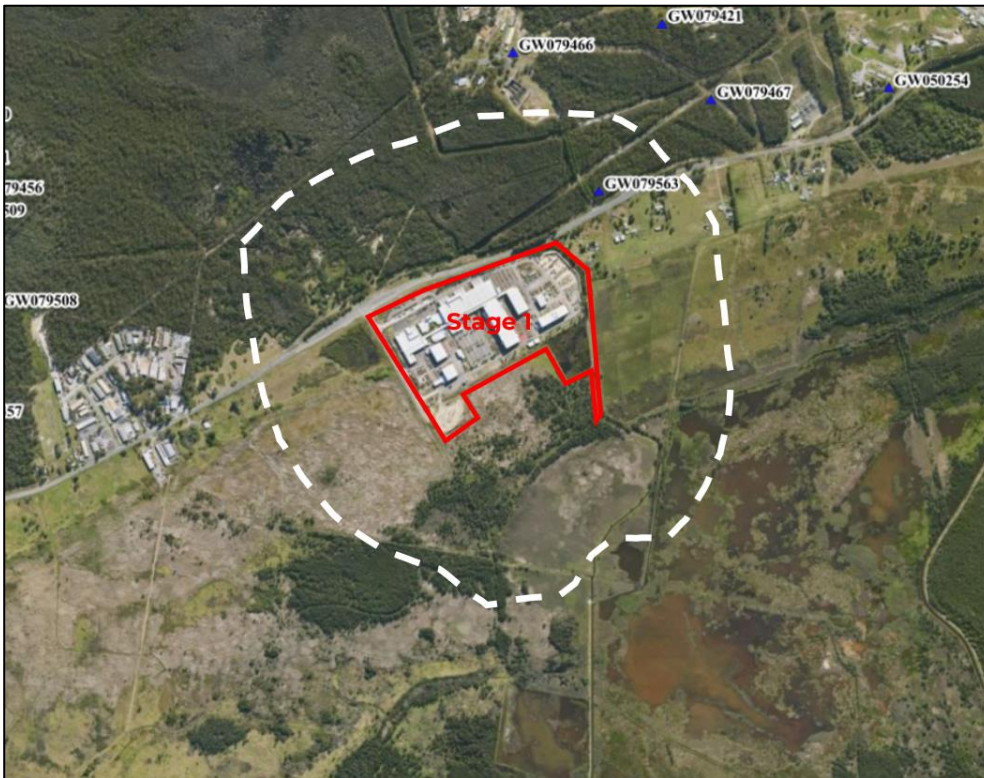
Figure 4: Registered groundwater bores relative to Stage 1 boundary. 500 m buffer shown in white
