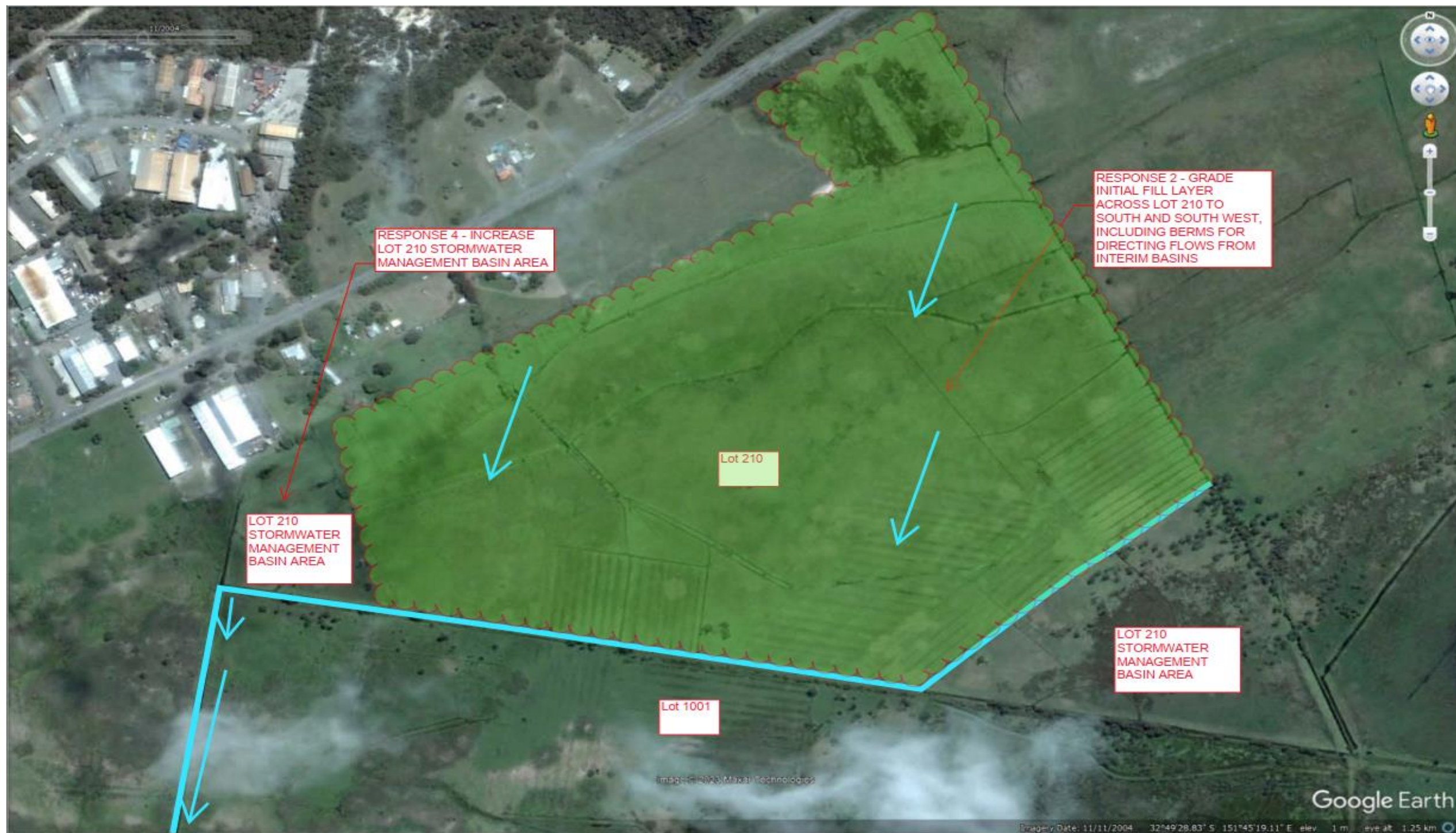
Figure 3: Response 2 (for TARP#1 on Page 1) - Extent of proposed initial fill layer, graded towards the south and southwestern boundaries of Lot 210
