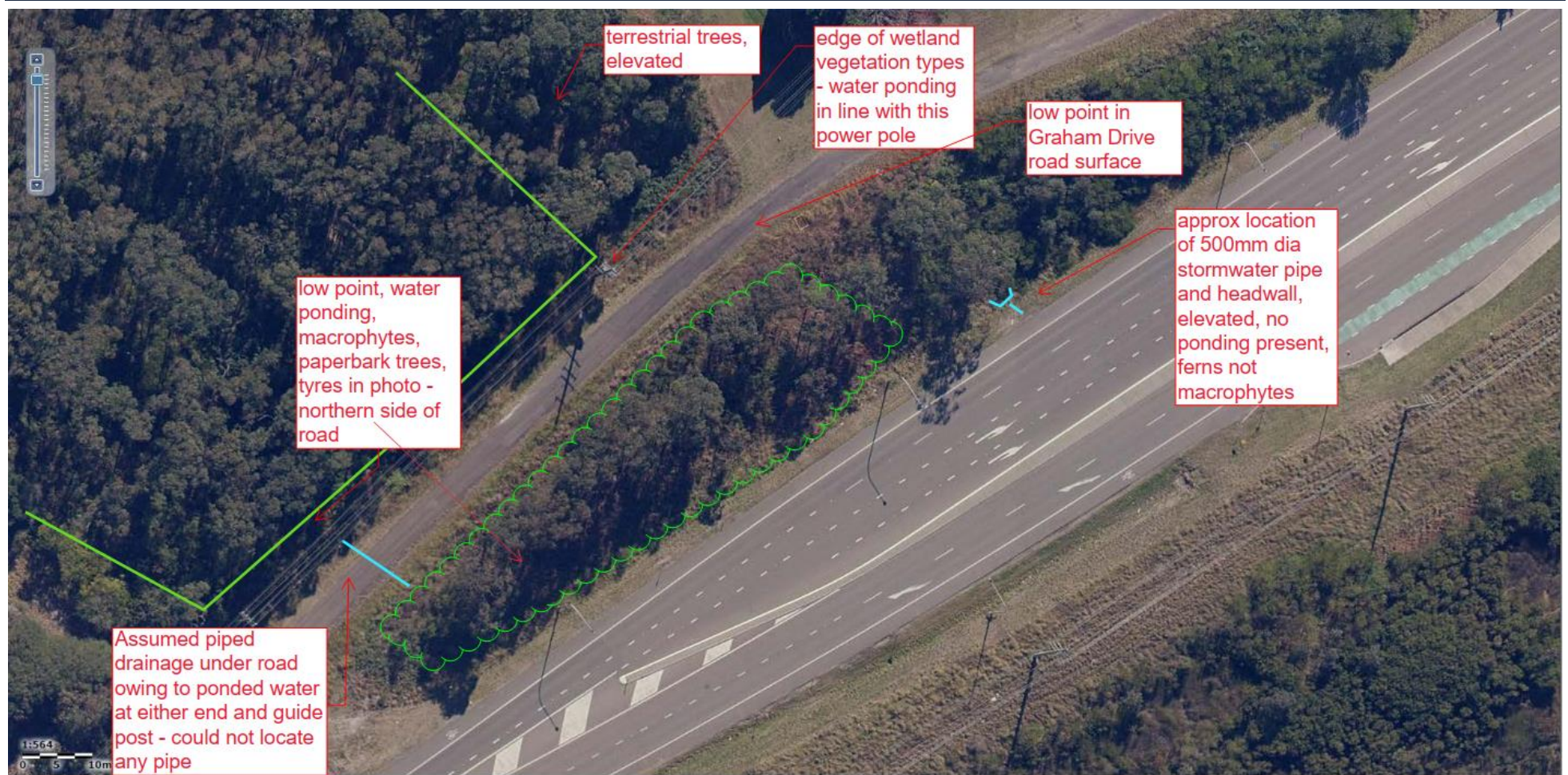
Figure 3.4 - Site observations of drainage characteristics at Graham Drive and Tomago Road just north of the development site
